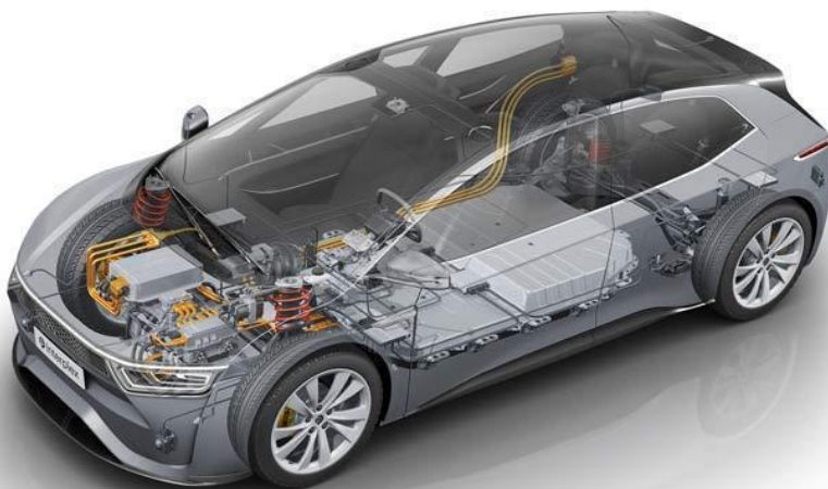
Figure 1. An overview of a typical EV architecture
